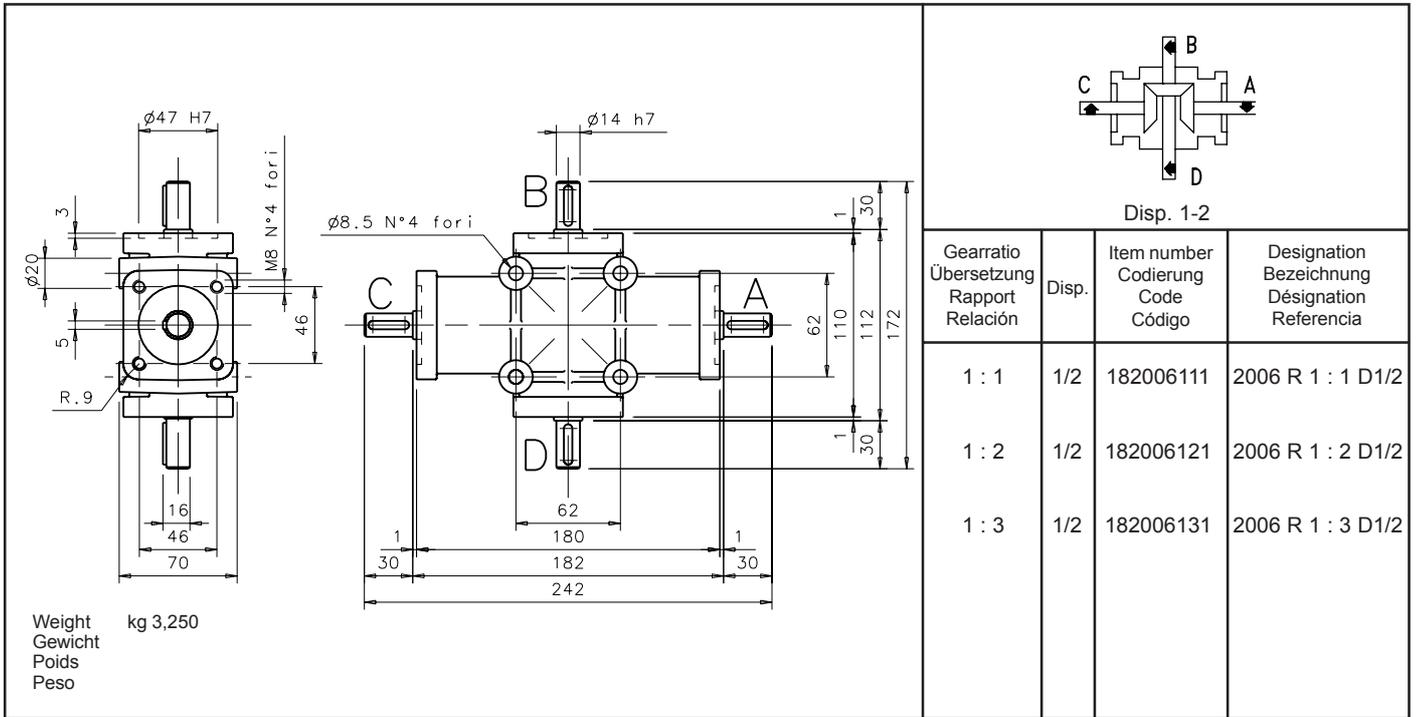
**3-way independent shaft angular transmission unit**
