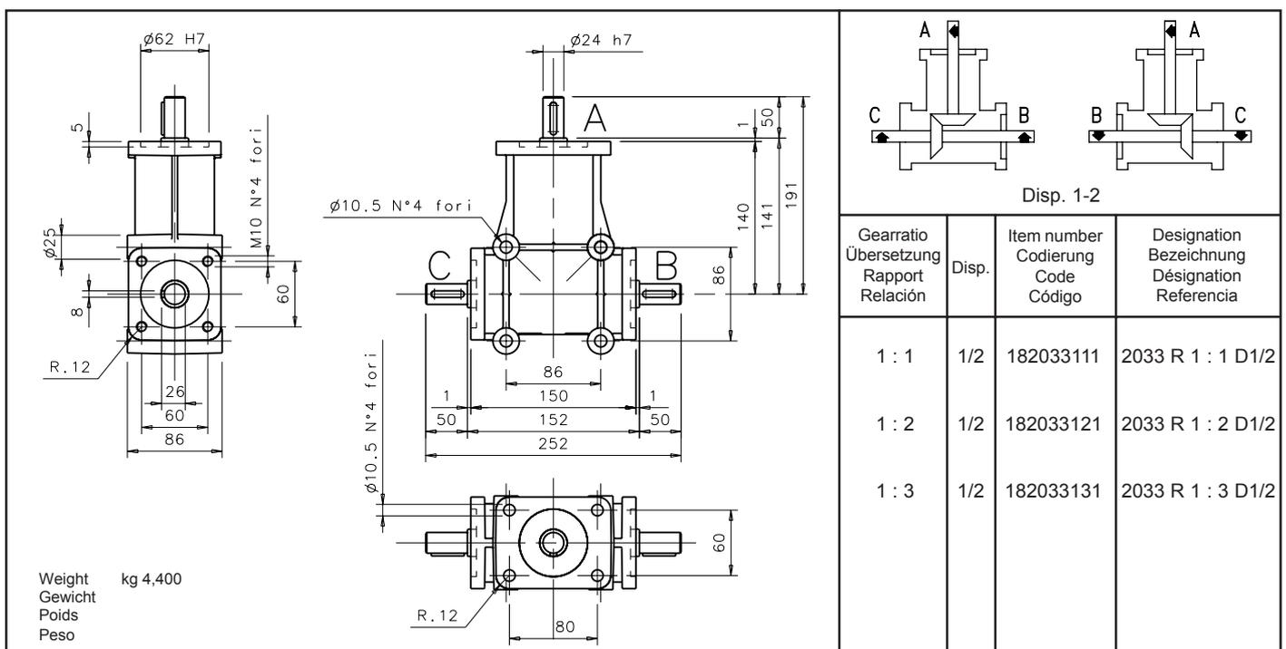
**3-way angular transmission unit with hollow output shaft**
