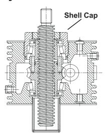
Sym-metric actuators are available with anti-backlash nuts for applications where a reversal of loading from tension to compression is encountered.
