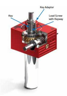
The Anti-Rotation feature for translating screw jacks stops the lead screw from rotating without the need for end fixing. This is done by keying the lead screw. However the keyway in the screw will cause slightly greater than normal wear on the internal threads of the worm gear.
